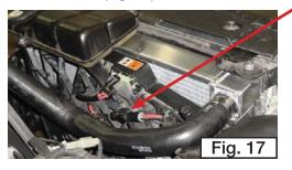
21. Attach the inlet and outlet hoses, and transmission lines (if an automatic car) to the radiator.
